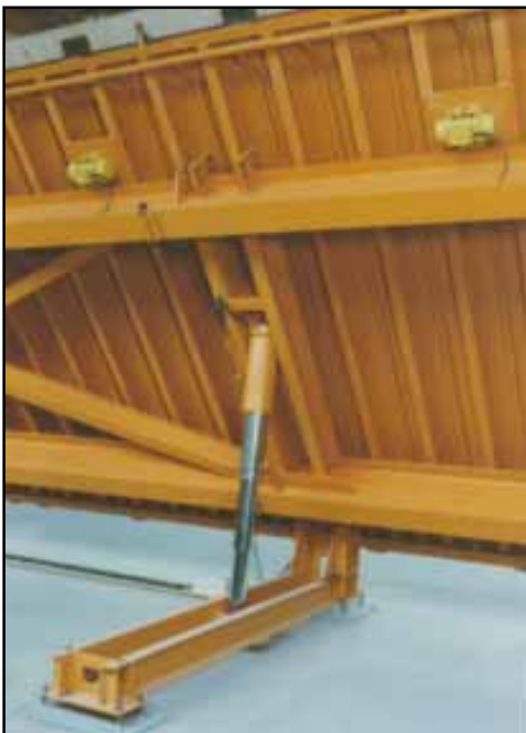
Tilting table with BRECON LICENCE BOSCH external vibrators 18 220
