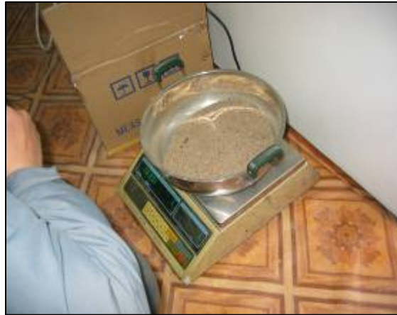
5 Re-weigh to ensure that there has been no change, i.e. material is in oven dried condition
